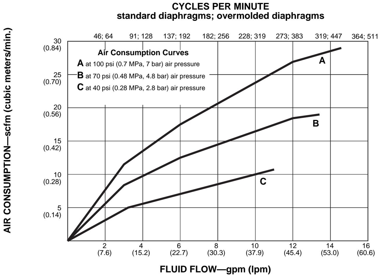
To find Pump Air Consumption (scfm or m<sup>3</sup>/min) at a specific fluid flow (gmp/lpm) and operating air pressure (psi/MPa/bar):
